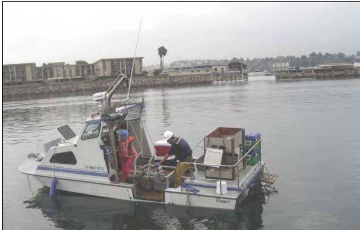
Figure 2. Van Veen grab sampling on the RV Waterline in Marina del Rey Harbor.
