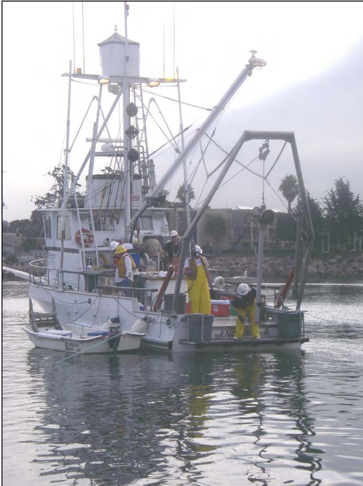
Figure 1. Vibracore sampling on the RV Early Bird II in Marina del Rey Harbor.
